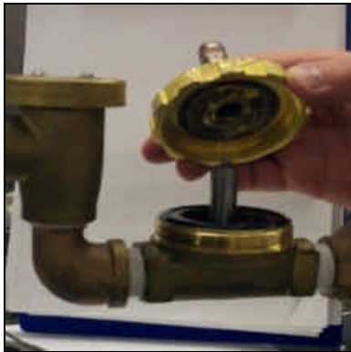
Removing the valve bonnet
